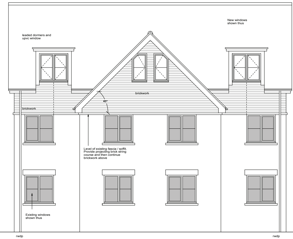
front / north elevation
